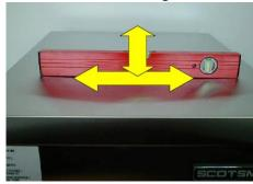
Level the unit in both directions, front to rear and right to left using the adjustable feet on the storage bin.
