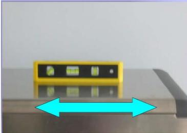
❖ Level the unit in both directions, front to rear and right to left side using the adjustable feet.
