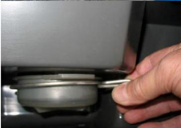
❖ Make sure the plug and spring are in place in the storage bin.
