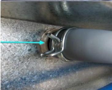
❖ Connect the water drain flexible hose supplied with the machine to the water drain fitting situated on the back of the machine using the clamp.
