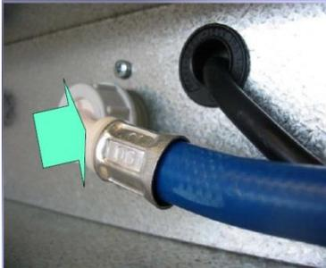
❖ Connect the water inlet hose provided with the ice machine to the water inlet valve situated on the back of the machine and connect the other end of the inlet hose to the water supply (3/4" male tread tap).
