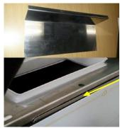
Place the metal bracket that holds the ice level control between the machine and the bin in line with the opening of the ice chute.
