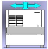
Level the unit in both directions, front to rear and right to left using the adjustable feet on the storage bin. 4)
