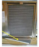
Remove the air baffle plate from the back of the unit.
