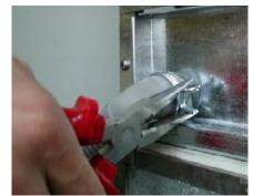
Connect the water drain flexible hose supplied with the machine to the water drain fitting situated on the back of the machine using the clamp.
