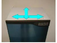
Level the unit in both directions, front to rear and right to left side using the adjustable feet on the storage bin.
