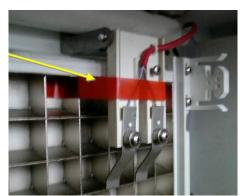
Remove the adhesive tape holding the ice thickness sensor to the evaporator plate.
