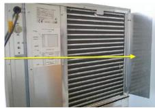
Install the metal baffle plate on the back side of the machine to minimize the possible recycling of hot air through the right side louver panel.
